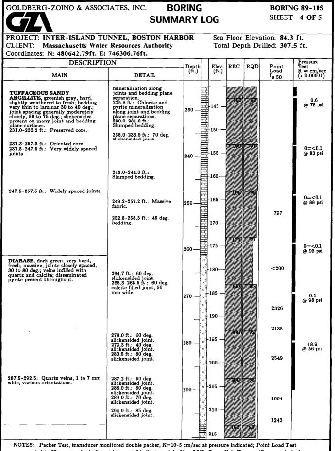
corrected to 55 mm standard, diametric except \* indicates axial. \*\* = SOIL, Down Hole Hammer/Recovery in inches.
