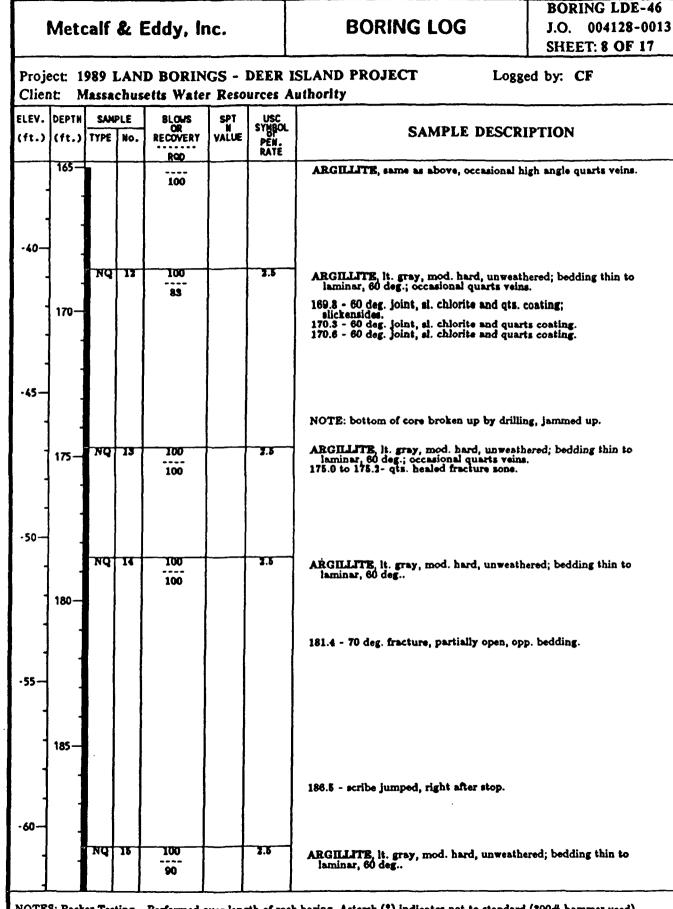
NOTES: Packer Testing - Performed over length of rock boring. Astersk (\*) indicates not to standard (300# hammer used). Preserved core 10.2 ft. Insitu testing 6 ft. away in LDE-46A. PMT- Menard Pressuremeter Test.
