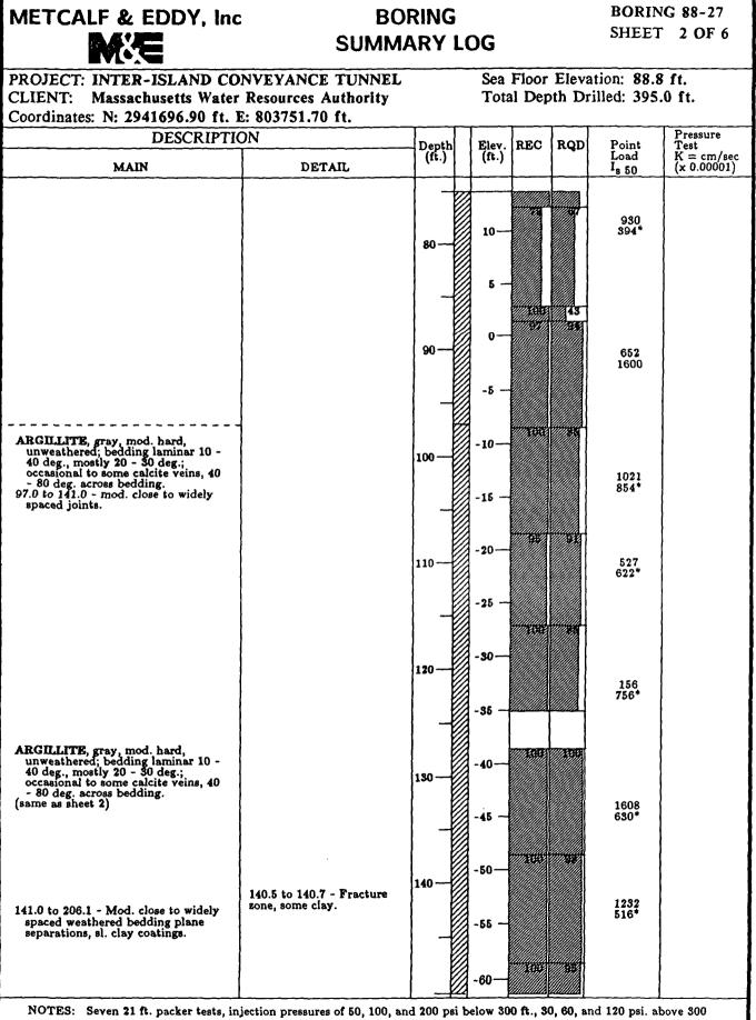
ft.; Point Load tests were diametral, \* indicates test perpendicular to bedding, + indicates axial.
