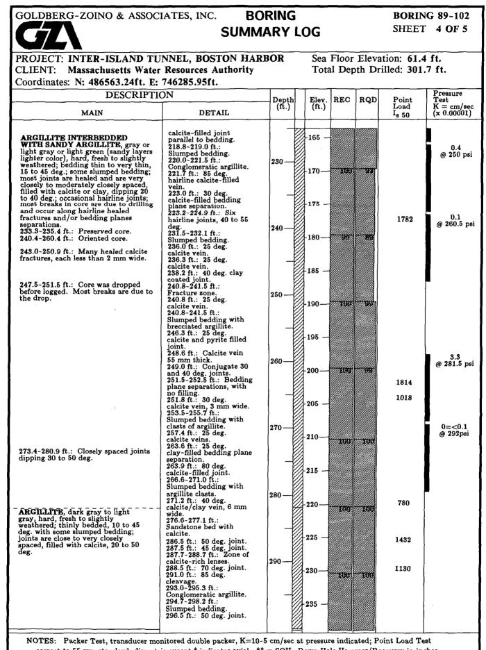
correct to 55 mm standard, diametric except \* indicates axial. \*\* = SOIL, Down Hole Hammer/Recovery in inches.
